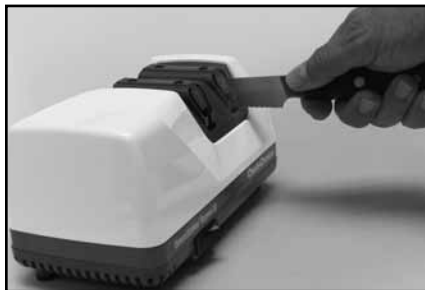
Figure 9. Sharpen serrated blades only in Stage 2. (See instructions.)
